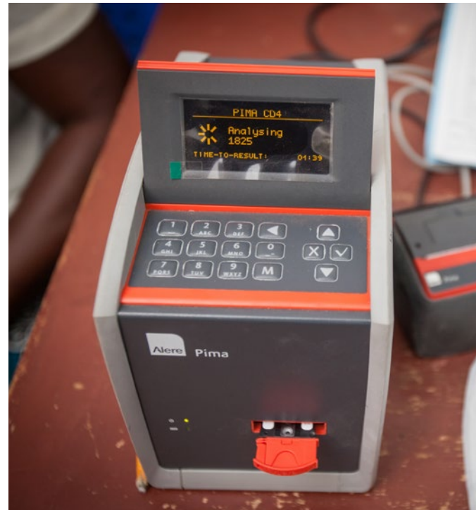
A NURSE OPERATES A PIMA CD4 TESTING MACHINE AT A HEALTH CENTER LILONGWE, MALAWI
